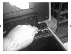
**STEP 5:** Using a T-20 socket, remove the pair of bolts at the top corners of the storage bucket.
